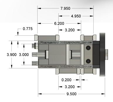
4 - Hardened steel jaws feature serrated, step and flat sides
